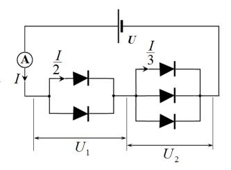
graphs. When connected in series the total voltage is the sum of the stresses in some parts of the circuit, so
