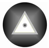
Since the source has, albeit small, but finite dimensions, the image of the triangle is to be slightly blurry, i.e. bordered by a semi-illuminated strip (border). The width of this strip is approximately equal to  $\Delta r \approx 3r_1 = 3$  mm. It can be imagined that each source point gives an image in the form of a triangle, these images are displaced relative to each other by the twice displacement of the source points.
