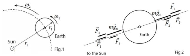
In Figure 2:  $mg_0$  is the force of gravitational attraction to the Earth;  $F_1$  is the centrifugal force due to the rotation of the Earth around its own axis;  $F_2$  is the force of gravitational attraction to the Sun;  $F_3$  is the centrifugal force due to the motion of the Earth around the Sun.
