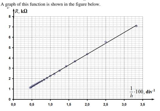
The parameters of this linear dependence, calculated by the mean square method  $a = (210 \pm 3) k\Omega \cdot div$
